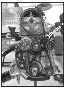
FIGURE 69. TIMING BELT A TENSION SIDE
