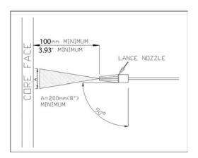
FIGURE 5. PRESSURE WASHER NOZZLE POSITIONING
