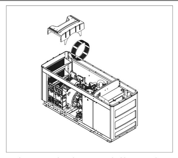
FIGURE 87. REMOVAL OF TERMINAL BOX COVER AND DOME
