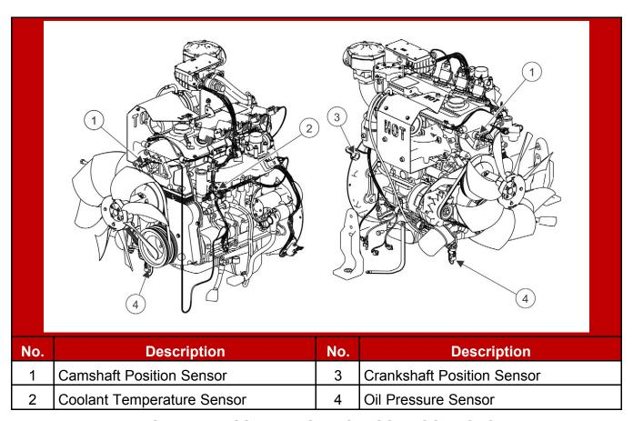
FIGURE 27. QSJ2.4 ENGINE SENSOR LOCATIONS
