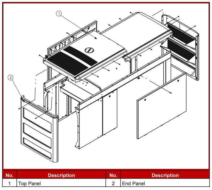
FIGURE 6. ENCLOSURE END PANEL REMOVAL
