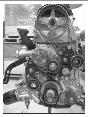
FIGURE 82. CRANKSHAFT BOLT AND WASHER
