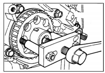
FIGURE 83. CRANKSHAFT SPROCKET REMOVAL
