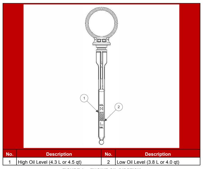
FIGURE 3. ENGINE OIL DIPSTICK
