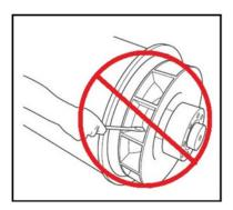
FIGURE 96. DO NOT ROTATE ROTOR USING FAN
