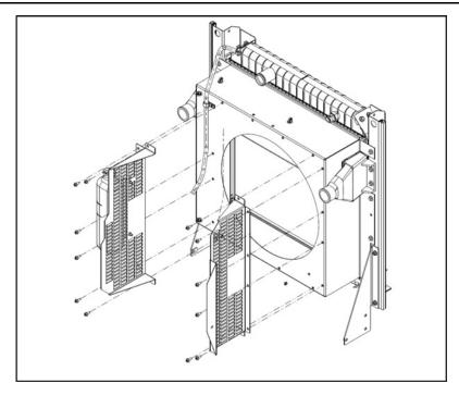
FIGURE 40. REMOVE FAN COMPONENTS
