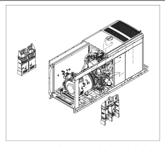
FIGURE 91. REMOVE TERMINAL BOX MOUNTING BOLTS
