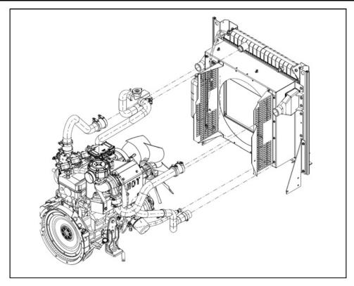
FIGURE 39. REMOVE CONNECTIONS
