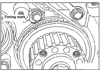
FIGURE 67. CRANKSHAFT SPROCKET AND FRONT CASE TIMING MARKS
