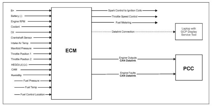
FIGURE 11. ECM INPUTS AND OUTPUTS
