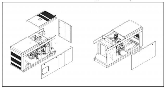
FIGURE 38. ENCLOSURE DOOR REMOVAL
