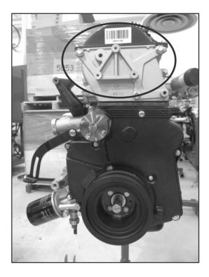
FIGURE 55. TIMING BELT UPPER COVER REMOVAL
