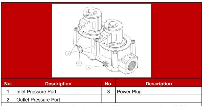
**Note:** Test port threads are G-1/8" and not 1/8" NPT. For test purposes only, a 1/8" ISO male to 1/8" NPT female adapter may be used.
