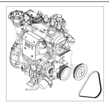
FIGURE 53. WATER PUMP, FAN, AND BATTERY CHARGING ALTERNATOR BELT
