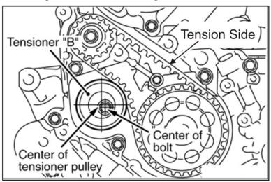
FIGURE 75. TENSIONER PULLEY CENTER
