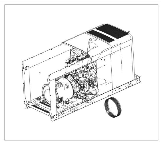
FIGURE 94. ALTERNATOR FAN GUARD (WITH DETAIL)
