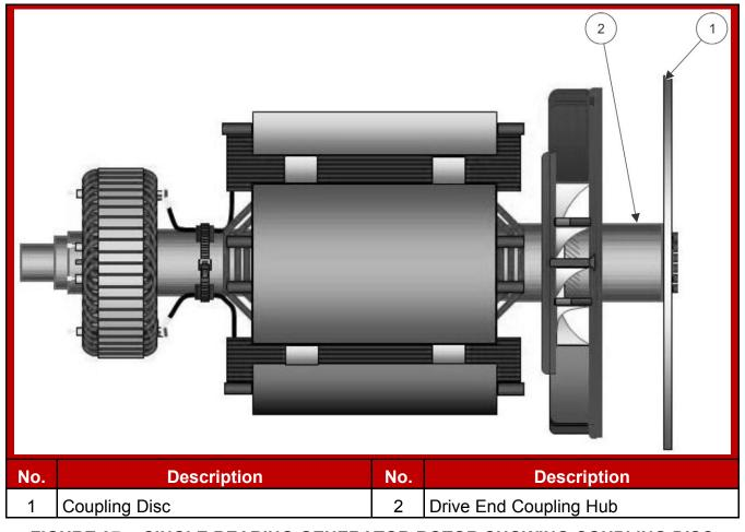
FIGURE 97. SINGLE BEARING GENERATOR ROTOR SHOWING COUPLING DISC BOLTED TO DRIVE END COUPLING HUB (AT RIGHT)
