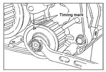
FIGURE 68. OIL PUMP SPROCKET AND MATING TIMING MARKS
