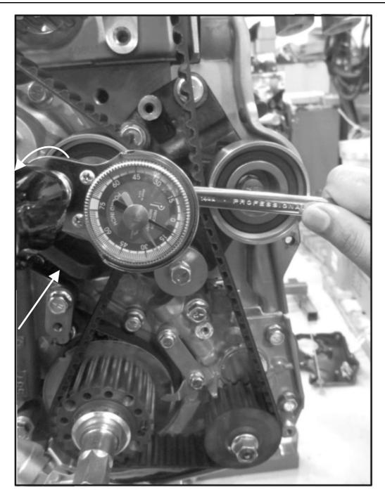
FIGURE 72. AUTOTENSIONER WITH SOCKET WRENCH (WITH BELT TENSIONING ARM)
