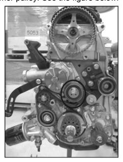
FIGURE 62. TENSIONER PULLEY
