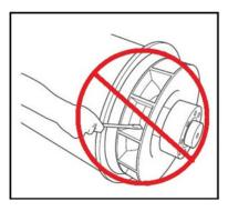
FIGURE 93. DO NOT ROTATE ROTOR USING FAN
