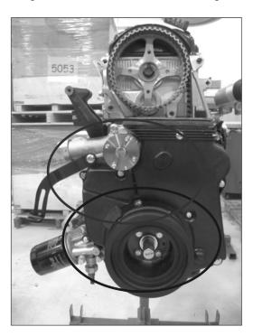
FIGURE 57. TIMING BELT LOWER COVER REMOVAL
