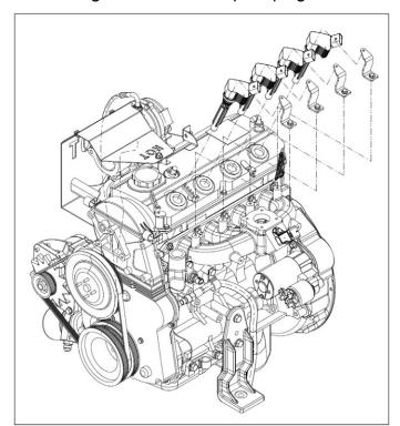
FIGURE 54. IGNITION COILS AND SPARK PLUGS
