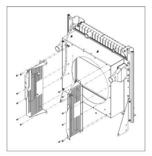
FIGURE 51. FAN GUARD REMOVAL
