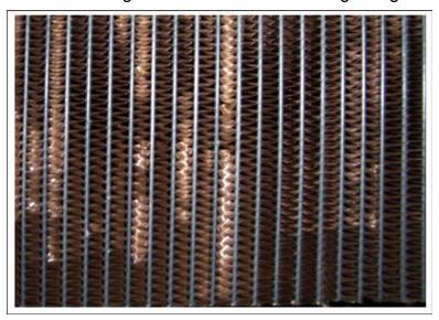
FIGURE 7. FINS DAMAGED BY COMPRESSED AIR AT ACUTE ANGLES TO CORE FACE
