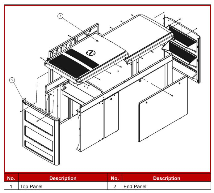
FIGURE 48. ENCLOSURE END PANEL REMOVAL
