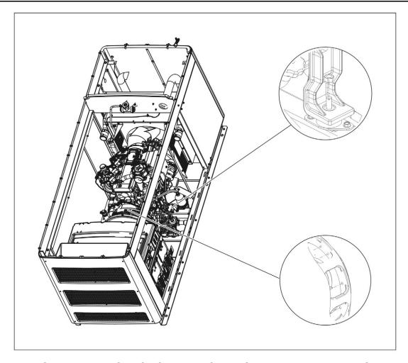
FIGURE 88. DISENGAGEMENT OF ENGINE AND ALTERNATOR
