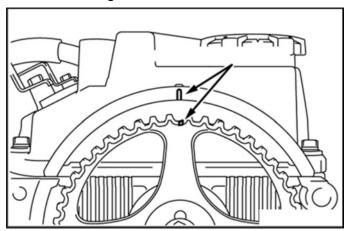
FIGURE 66. CAMSHAFT SPROCKET AND ROCKER COVER TIMING MARKS
