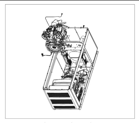
FIGURE 89. ENGINE REMOVAL
