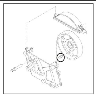
FIGURE 81. CAMSHAFT PIN MOUNTING
