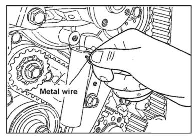
FIGURE 73. REMOVE METAL WIRE
