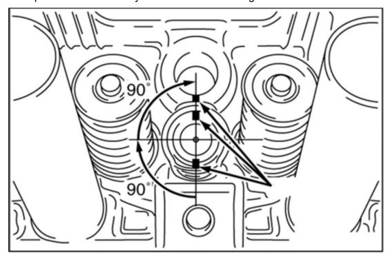
FIGURE 80. PAINT MARK ALIGNMENT
