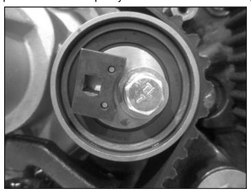
FIGURE 71. AUTOTENSIONER WITH SOCKET WRENCH
