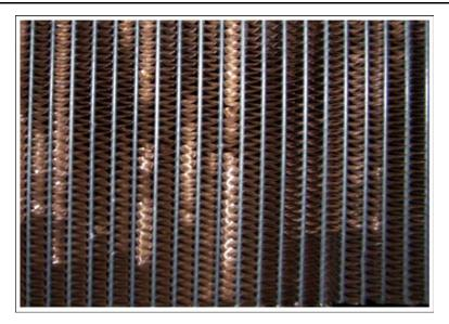
FIGURE 4. FINS DAMAGED BY PRESSURE WASHING AT ACUTE ANGLES TO CORE FACE
