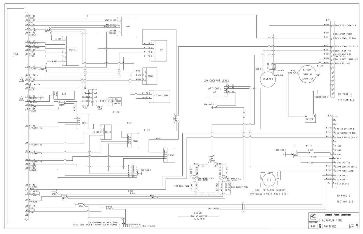
FIGURE 105. WIRING DIAGRAM (SHEET 2 OF 7)
