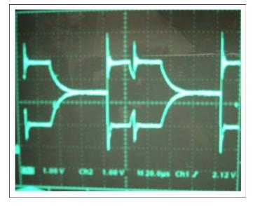
FIGURE 26. CAN DATALINK: BAD SIGNAL
