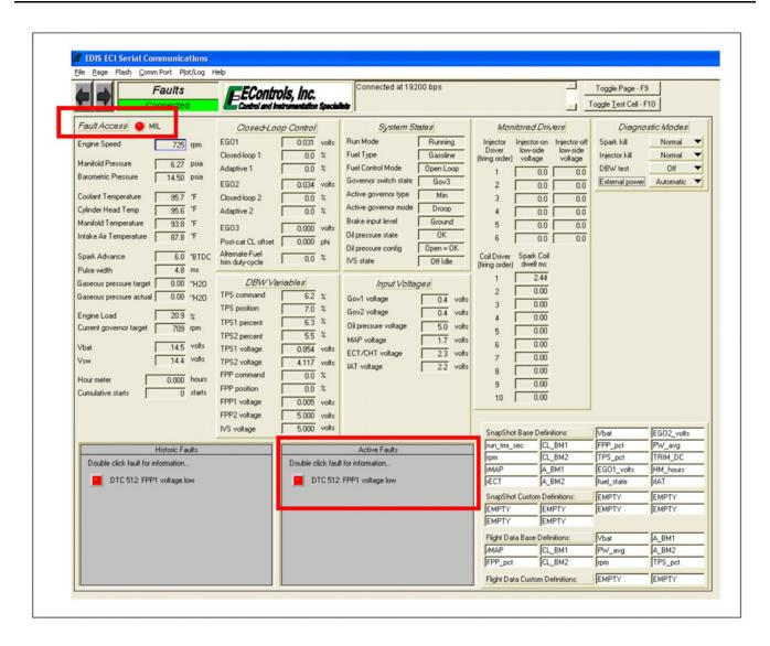
FIGURE 19. FAULTS PAGE WITH ACTIVE FAULT MESSAGE
