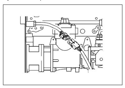
FIGURE 10. CHECK HARNESS CONNECTIONS
