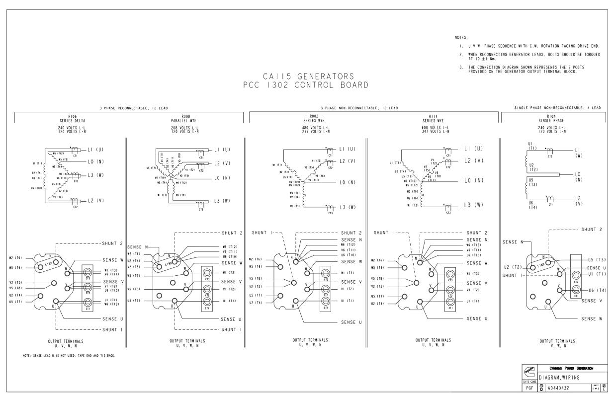
FIGURE 111. ALTERNATOR RECONNECT, WIRING DIAGRAM FOR AW1 (SHEET 1 OF 1)
