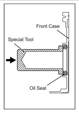
FIGURE 84. CRANKSHAFT FRONT OIL SEAL
