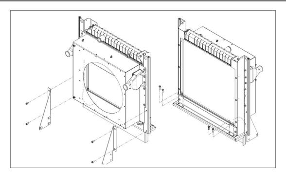
FIGURE 42. SUPPORT BRACKETS AND BOTTOM BRACKET
