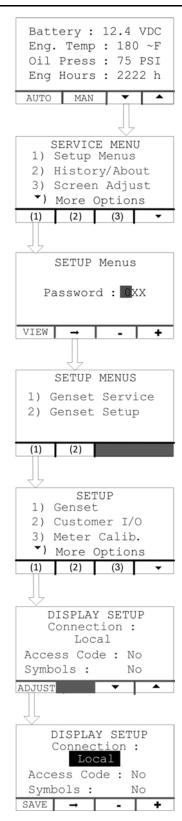
FIGURE 98. DISPLAY SETUP MENU NAVIGATION
