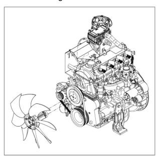
FIGURE 52. FAN REMOVAL
