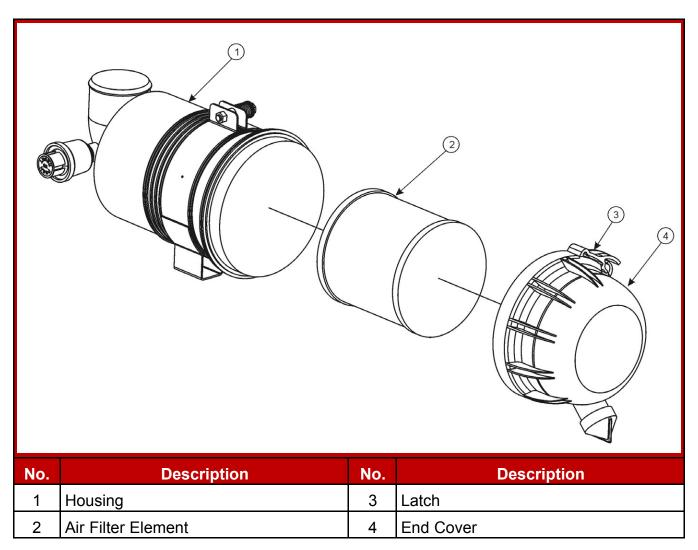
FIGURE 9. EXAMPLE OF HEAVY DUTY AIR CLEANER
