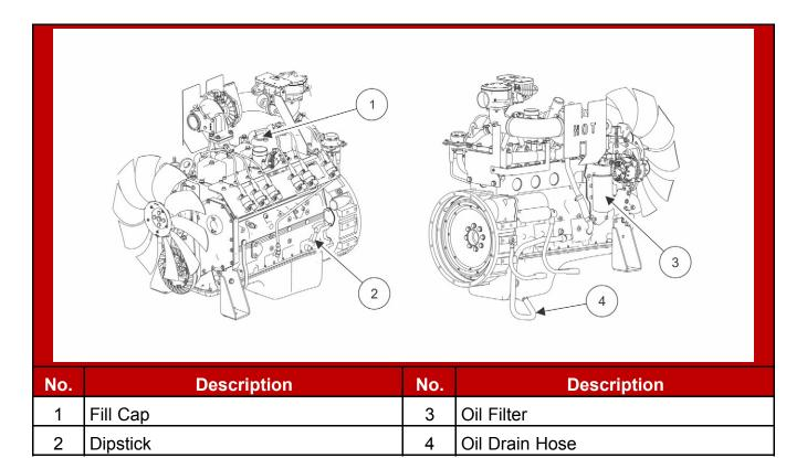
FIGURE 2. ENGINE OIL COMPONENTS
