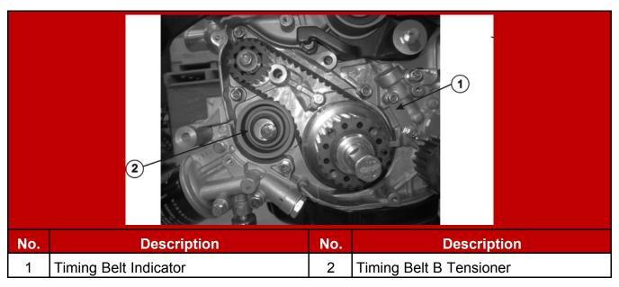
FIGURE 61. TENSIONER PULLEY
