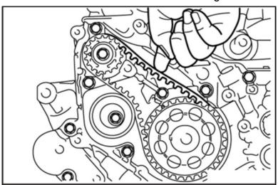
FIGURE 77. CHECK TIMING BELT TENSION
