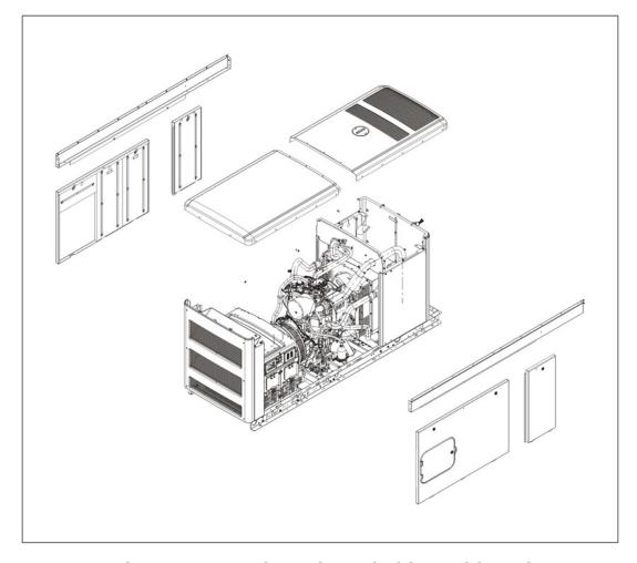
FIGURE 85. REMOVAL OF ENCLOSURE COVERS
