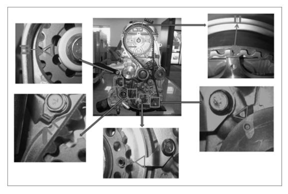
FIGURE 58. TIMING MARK ALIGNMENT
