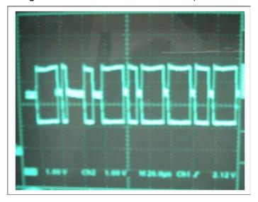
FIGURE 25. CAN DATALINK: GOOD SIGNAL
